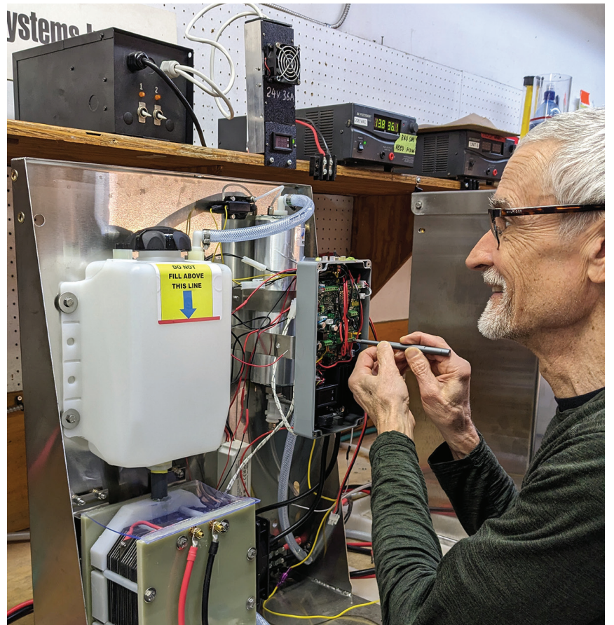
Technician David Butcher fine tunes the hydrogen/oxygen gas production circuitry
