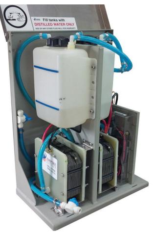
The Empire Hydrogen system is offered in 12- and 24-volt versions, respectively suiting on- or on/off-road and off-road power units. Charges are applied to the system's stainless steel plates, which harbor distilled water and potassium hydroxide. An electric current breaks the water molecules into a 2:1 mixture of  $H_2$  and  $O_2$  gases, which serve as accelerants when injected into the fuel combustion stream.
