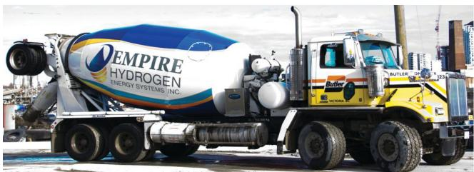
Across its nearly 40-mixer fleet, Butler Concrete and Aggregate is tracking diesel and diesel exhaust fluid savings attributable to the Empire Hydrogen Fuel Enhancement System, mounted between the drum and water tank. The lead McNeilus mixer bears on a Western Star 4800 Twin Steer, with Detroit DD 13 power and Eaton UltraShift automated manual transmission.
