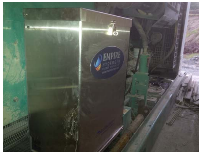
Empire Hydrogen on a Butler Concrete Generator
