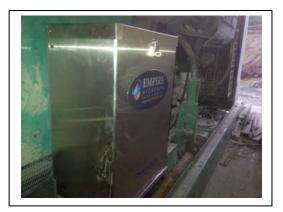
Empire's Bill Campbell closed this contract and has worked with Butler's full team of mechanics to create a product for the unique requirements of concrete trucks which do not have standard shock absorber systems. We will be installing cable springs under each unit to absorb the rough conditions faced on a daily basis. We can use this knowledge for future installations on other off road equipment.
