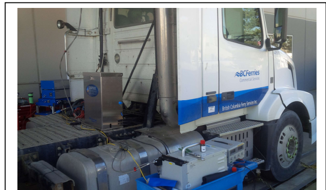
The Class 8 Fuel Enhancement System on a larger BC Ferries Volvo VNL 600, on the BCIT dynamometer
