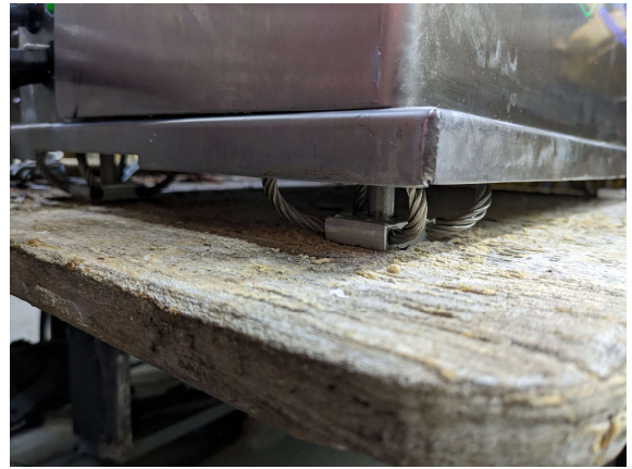
Cable springs provide shock absorption when the Empire Hydrogen Fuel Enhancement System is subjected to enormous mechanical stress.
